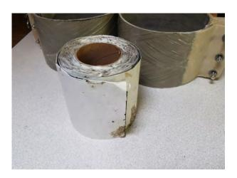
5. Cut a length of the butyl rubber gasket material from the supplied bulk roll. Size the cut gasket length to completely wrap around the duct diameter plus an overlap of approximately two inches (2").
